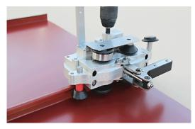
**2.** Position the ACCUSEAMER with the red marked Wheels over the Seam and start seaming.
