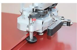
Place the ACCUSEAMER over the Seam and make sure that the angled front Guidewheel is under the
